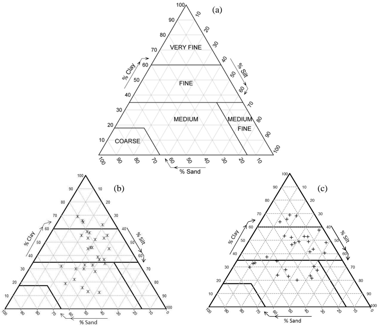
625 **Figure 2:** FAO triangle (FAO, 1990) of texture used (a), distribution of soil texture from samples used in this
