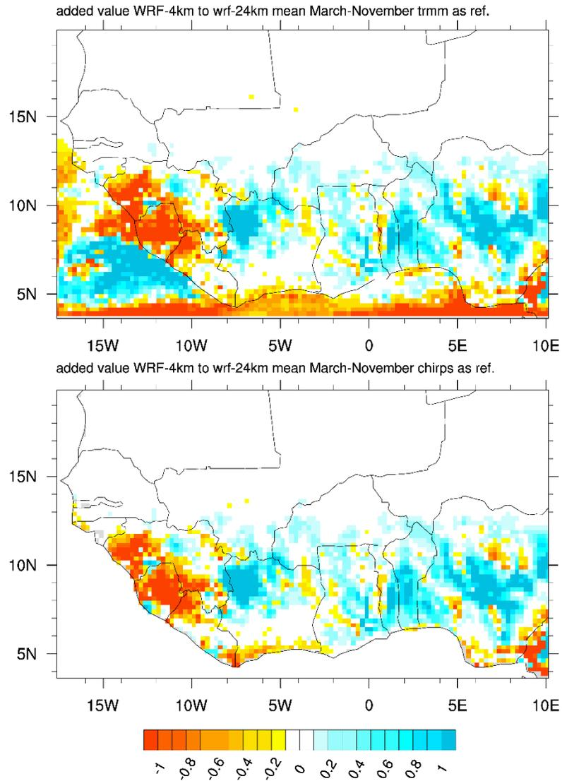
**Fig. 3** Added value of high resolution (wrf-4km) simulation to coarse resolution (wrf-24km): on top computed using TRMM as reference dataset and the bottom computed using CHIRPS dataset as the reference.
