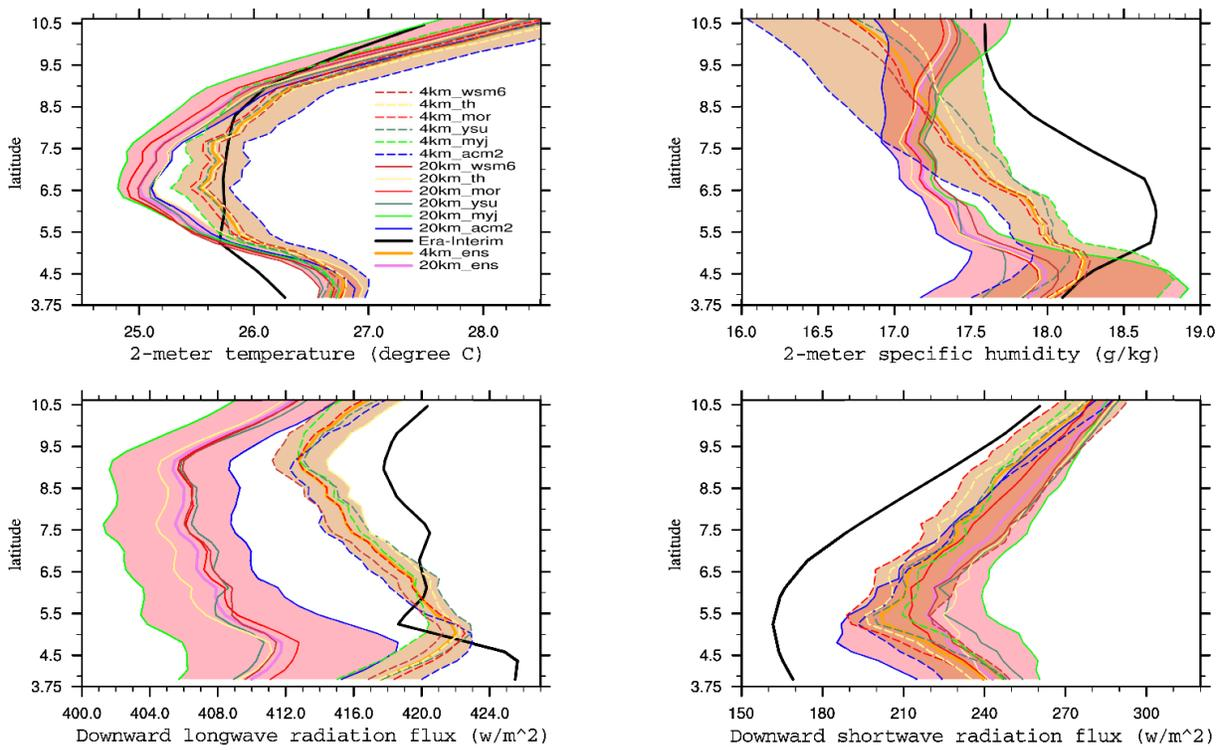
**Fig. 10** Meridional evolution of 2-meter temperature, specific humidity, downward shortwave and longwave radiation fluxes from wrf-20km and 4km ensemble group members and from Era-interim data set. All the values are averaged from 10W to 5 E. The pink and orange coloured areas mark the range of value respectively with wrf-24km and wrf4km.
