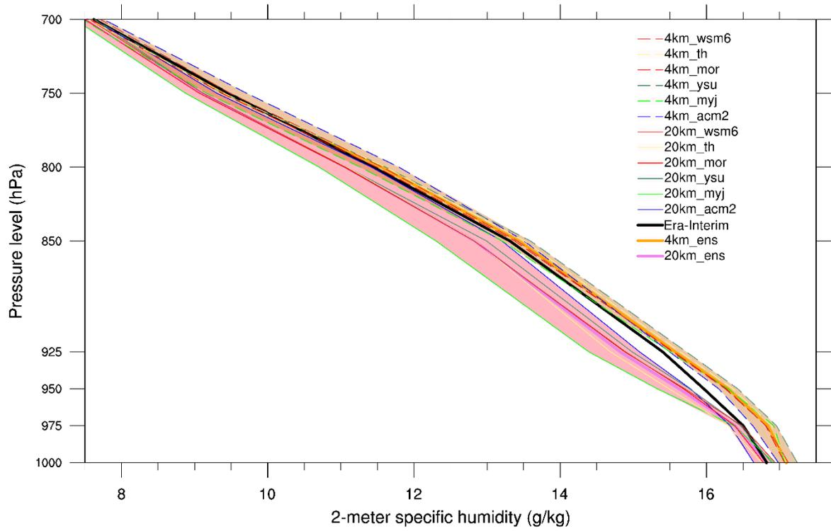
**Fig. 9** Vertical profiles of specific humidity from wrf-20km and 4km sub-ensembles group members and Era-interim data set. All the values are averaged from 10W to 5E. The pink and orange coloured areas mark the range of value respectively with wrf-24km and wrf4km.
