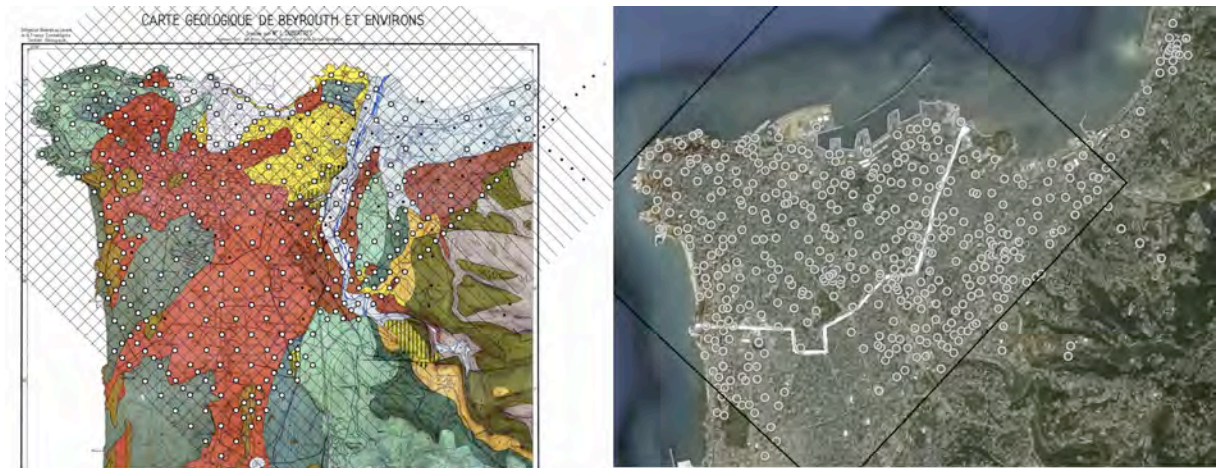
Figure 2. (Left) The initial 400m spacing grid of the ambient noise measurements sites. (Right) The effective measurements sites. The white continuous line represents the borders of Beirut municipality. The black rectangular delineates the area of the grid shown in the left image
