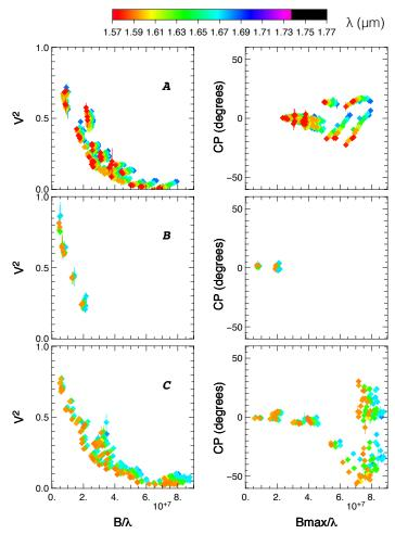
**Fig. 3.** Temporal representation on data taken on MWC158. The colours correspond to the wavelength. Dataset in V2 and CP. We notice strong differences in the CP between the epochs that may indicate variability.
