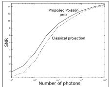
**Fig. 13.** Comparison of classical projection and Poisson proximity as a function of the number of photons ( $10^5$  photons  $\approx 1$  photon per pixel, on average).
