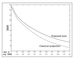
**Fig. 12.** Comparison of both projectors using the DR algorithm as a function of noise (noise level given in standard deviation and SNR).
