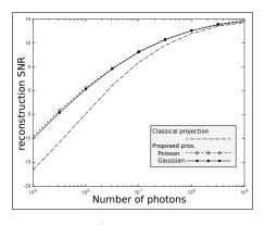
**Fig. 14.**  $SNR(x^+)$  as function of the number of photons in presence of a  $3e^-$  dark current.
