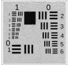
**Fig. 15.** Central  $250 \times 250$  pixels of the test chart recovered from 8 planes measurements using the proximity operator for sum-of-intensity measurements and back-propagated to z = 0.
