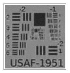
Fig. 6. Intensity of the estimated wave using the classical projection (noise standard deviation  $\sigma = 0.3$ ) backpropagated from  $z_A$  to  $z_0$ . SNR( $x^+$ ) = 6.37 dB.
