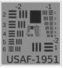
Fig. 7. Intensity of the estimated wave using the proposed proximity operator (noise standard deviation  $\sigma = 0.3$ ) backpropagated from  $z_A$  to  $z_0$ . SNR( $x^+$ ) = 7.60 dB.
