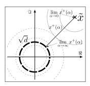
Fig. 1. Trajectory of  $x^+(\alpha) = \operatorname{prox}_{\alpha f}(\widetilde{x})$  as a function of  $\alpha$ .  $x^+(\alpha)$  follows the line where the level set of *f* (thin dashed circles) and  $|x - \tilde{x}|^2$  (thin circles) are tangent.
