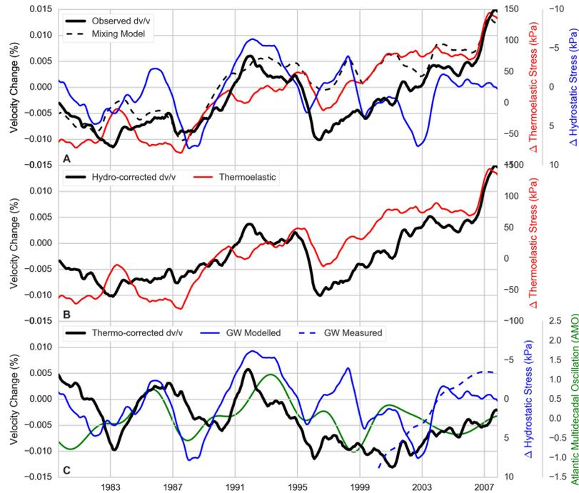
**Figure 5.** Observed  $dv/v$  and results of modeling. **(A)** Observed  $dv/v$  (black), modeled  $dp_i$  (red), modeled  $dp_h$  (blue) and Mixing model  $M = 0.5 * \alpha * dp_i - 0.5 * \beta * dp_h$  (dashed black); **(B)**  $dv/v + \beta * dp_i$  (“hydro-corrected  $dv/v$ ”, black) and  $dp_i$  (red). **(C)**  $dv/v - \alpha * dp_i$  (“thermo-corrected  $dv/v$ ”, black),  $dp_h$  from model (blue) or observed (dashed blue) and Atlantic Multidecadal Oscillation index (green).
