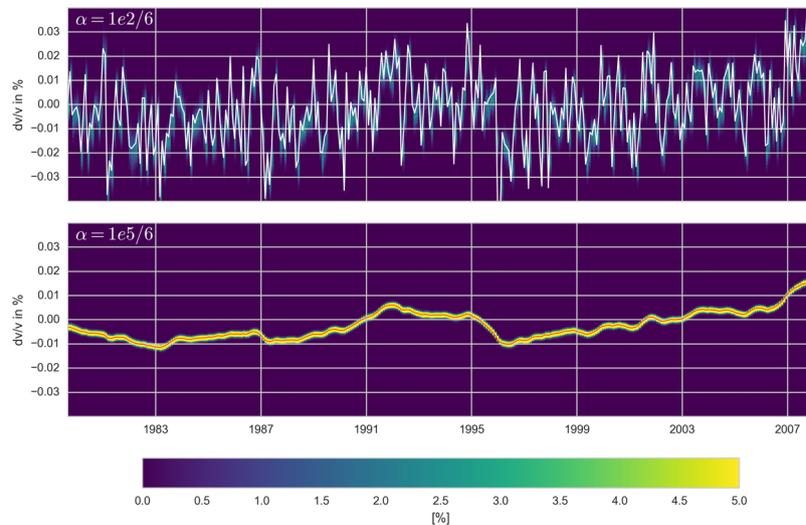
**Figure 10.** Inversion results using a bootstrap procedure. The color scale shows the percentage of spectra that fall into the  $dv/v$  pixel. The value computed with  $\alpha = 100$  (top) or  $100\,000$  (bottom) for the complete dataset (6 pairs) are shown in white (top) or red (bottom). The use of a smaller (larger)  $\alpha$  value induces a lighter (stronger) smoothing.
