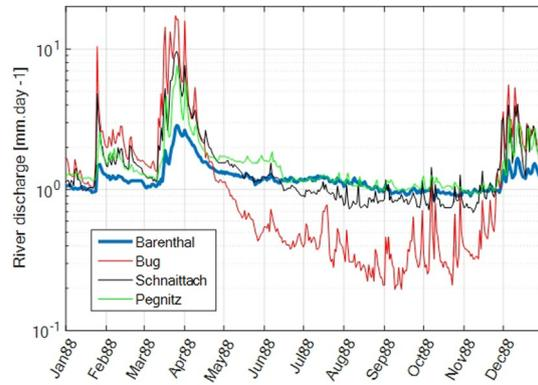
**Figure 13.** River discharge data for four discharge stations, for year 1988. Discharge can vary over several orders of magnitude, highlighting the integrated behavior of the catchment with respect to boundary conditions (P, E). Discharge variability in Bärenthal (blue line) is the smallest, suggesting a stronger control of groundwater to discharge.
