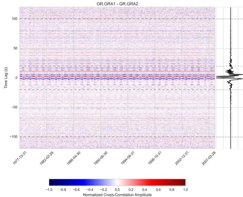
**Figure 8.** Monthly cross-correlation functions over 30 years for station pair “GRA1-GRA2”, colour coded by amplitude. The horizontal dashed lines indicate the part of the coda used in the  $dv/v$  calculation. The right panel shows a stack of all months.
