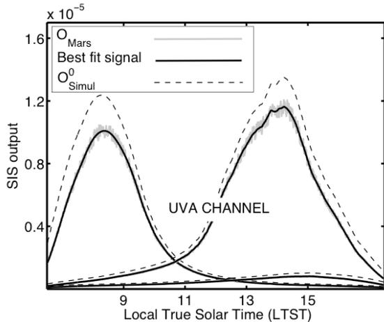
**Figure 2:** Comparison between  $O_{\text{Mars}}$  signals computed for  $\tau^{UVA}=0.7$ ,  $m^{UVA}=1.5+i0.02$  and  $r_{\text{eff}}=1.4 \mu\text{m}$  (grey solid lines), and those simulated using the retrieved (black solid line) and a priori (black dashed line) values of the free parameters illustrated in first line of **Table 1**.
