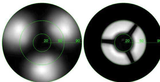
**Figure 1:** Measured FOV of SIS'16 (left) and ODS (right). White and black areas correspond to 100 and 0 % of transmission, respectively. The SIS FOV is employed using a total of three sensors oriented at different zenith angles while the ODS one using only one sensor and optical components.
