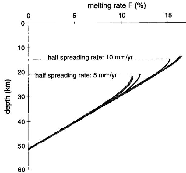
**Figure B1.** A comparison of melting rate versus depth curves obtained with our 1-D thermal and melting model (solid curves) and with the 2-D model of Bown and White [1994] (grey curves) for two values of the half spreading rate (5 and 10 mm/yr) and for a mantle temperature at solidus of 1300°C. Boundary conditions and melting parameters are the same as given by Bown and White [1994].
