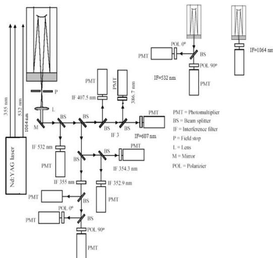
**Figure 1:** Block diagram of the system setup.
