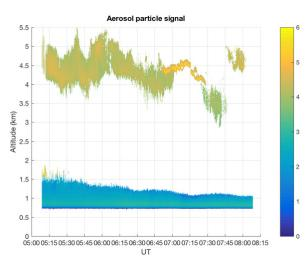
Figure 5: MARBLL range corrected signal @ 1064 nm (arbitrary units, SNR > 10) as a function of altitude from 5 UT to 8 UT (sunrise at 5:20 UT).
