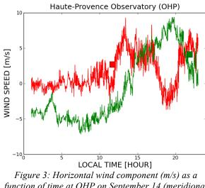
function of time at OHP on September 14 (meridional wind in red) and on September 16 (zonal wind in green). Continuous lines are the measurements from the ICOS mast (100 m above ground level), squares are MARBLL measurement at the same altitude.
