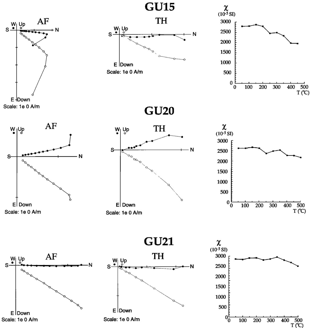
Figure 5. Zijderveld [1967] plot of stepwise demagnetization of two samples per flow (one with thermal and one with AF treatment) for the three sites also sampled by Briden *et al.* [1979]. See Figure 3 for convention of plots, and Table 4 for comparison of mean directions.
