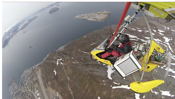
Figure 2. N_2 -Raman lidar embedded on ULA.
