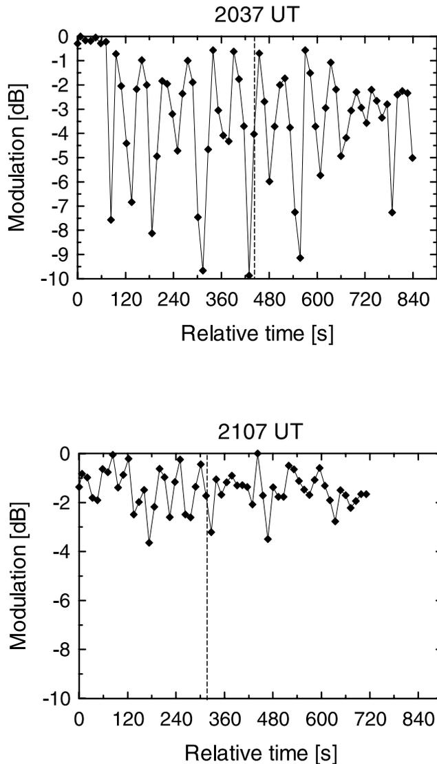
**Figure 2.** The modulation patterns for 2037 UT and 2107 UT events as seen with POLRAD experiment *Y* antenna (located in the plane perpendicular to the direction toward the Sun). Spacecraft coordinates were altitude 19,074 km, invariant latitude  $71.9^\circ$ , and MLT 22.00 for the 2037 case and 18,037 km,  $68.17^\circ$ , and MLT 22.55 for the 2107 case. Vertical dashed lines mark moments of MEMO data acquisition.
