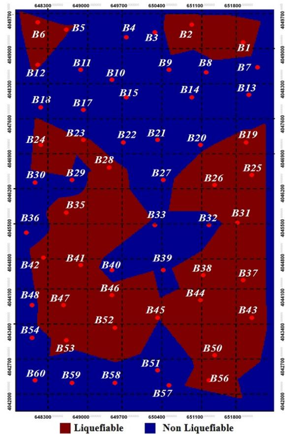
Fig. 7 Liquefaction microzonation of Babol by microtremor measurement
