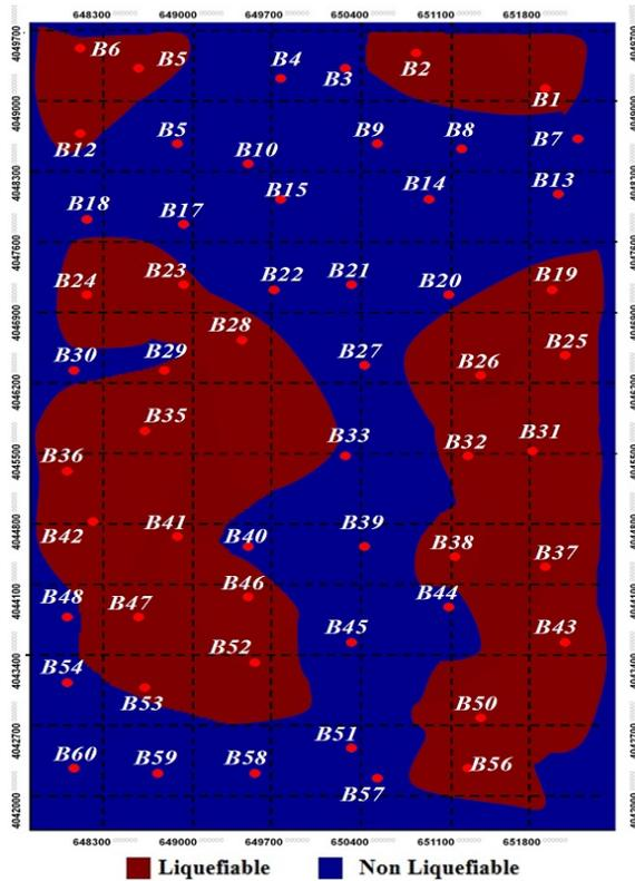
Fig. 8 Liquefaction microzonation of Babol by ANN
