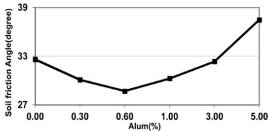
Fig. 5 International friction angle versus amount of alum
