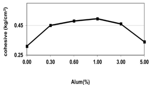
Fig. 4 Apparent cohesion for different percentages of additive
