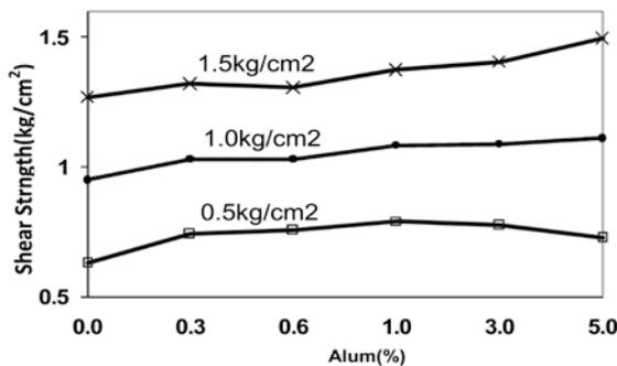
Fig. 6 Shear strength variations versus amount of alum
