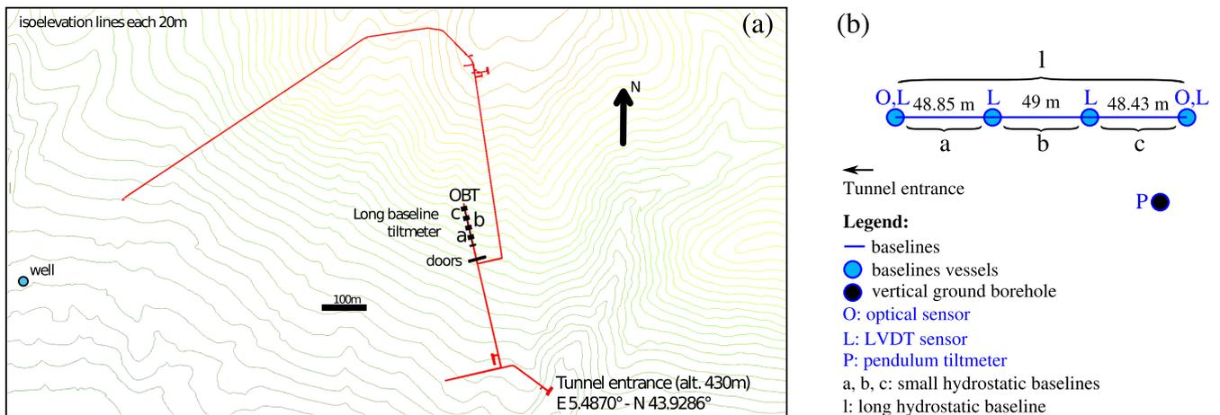
Figure 2. (a) Topography above the LSBB, galleries are indicated in red. Vertical deformations were measured at four points in order to provide tilt on a long-baseline tiltmeter of about 150 m and on three baselines of about 50 m. Piezometric data were measured from the well located outside, west of the LSBB. (b) Scheme of the tiltmeters location in the tunnel.
