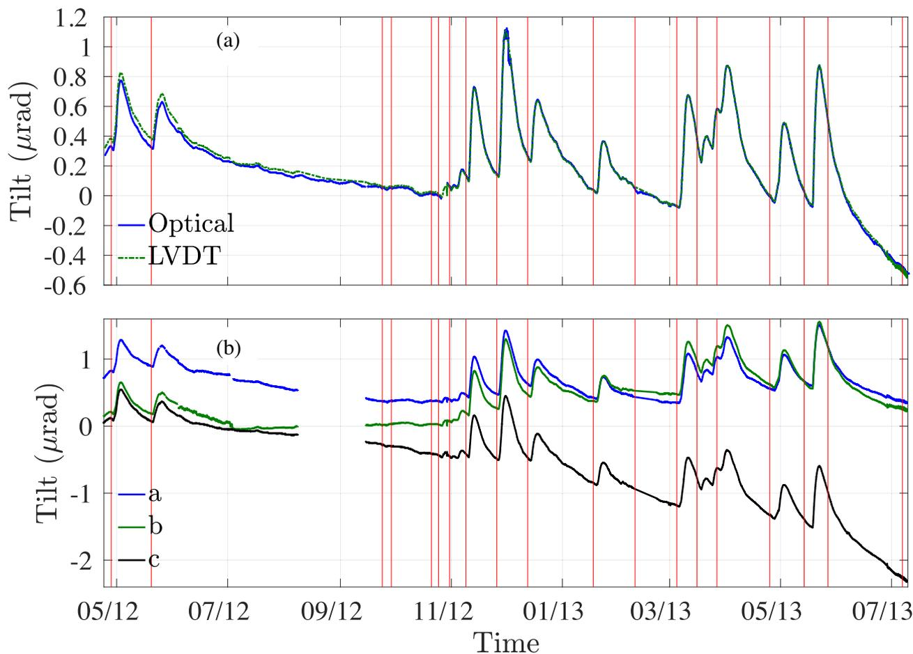
**Figure 5.** Comparison of the tilts measured with the different sensors. (a) Long-base tilt measured with optical and LVDT sensors. (b) Tilt measured with the smaller instruments a, b and c with LVDT sensors.
