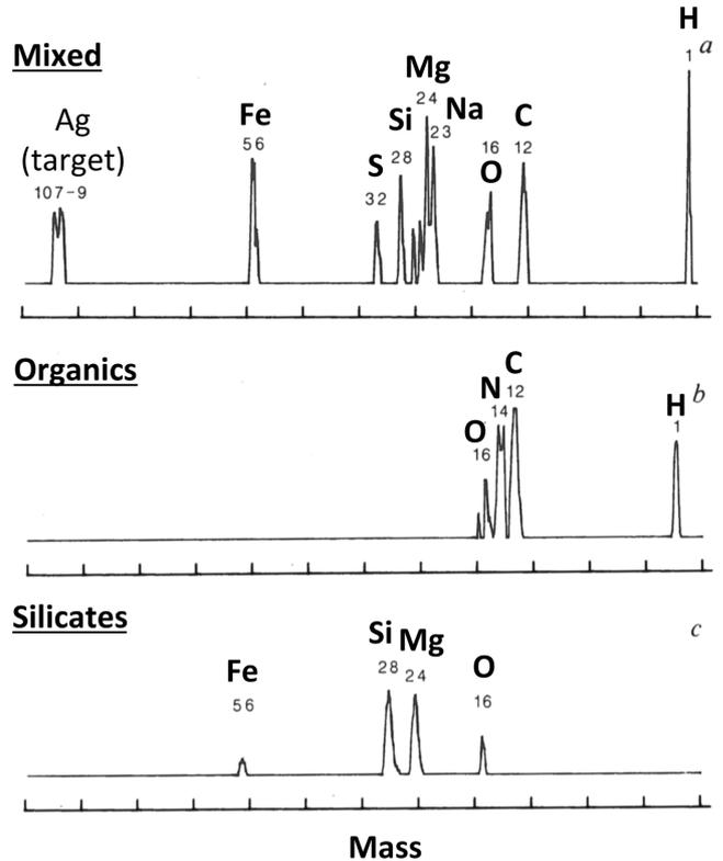
**Figure 1.** Typical mass spectra obtained by the PIA instrument (particle impact analyser), a mass spectrometer on the *Giotto* spacecraft (vertical log scale) (adapted from Kissel et al. 1986a). Proposed element identification has been added to the mass peaks for clarity. The mixed (a) and organics (b) types represent 80 per cent of the total number of spectra (see original article for details). Reprinted by permission from Macmillan Publishers Ltd: Nature, copyright (1986).
