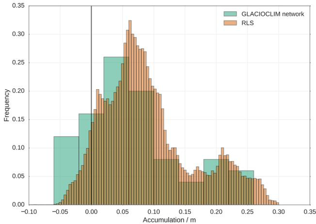
**Figure 11.** Distribution of the spatial variations of accumulation at Dome C observed by RLS (measured between 3 January and 5 December 2015) and the GLACIOCLIM network at 2 km from Concordia station (measured between 3 January and 18 November 2015).
