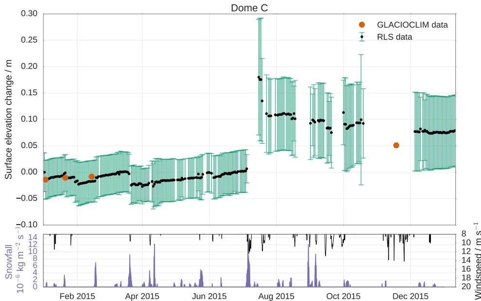
**Figure 4.** Evolution of the mean (black) and standard deviation (green) of the surface elevation change at Dome C in 2015 and January 2016 measured by the RLS. Orange points show the mean accumulation deduced from emergence measurements of the GLACIOCLIM 50-stack network. The reference is calculated so that the first GLACIOCLIM measurement (3 January 2015) equals the mean RLS snow elevation measured the same day.
