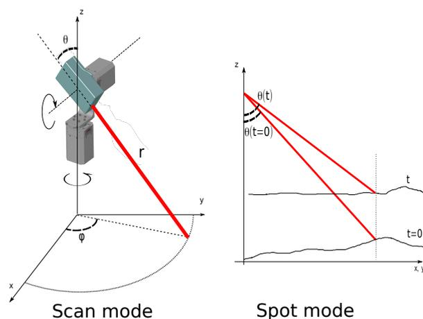
**Figure 1.** Principle of the scan mode and spot mode of the Rugged Laser Scan (RLS). The zenith angle  $\theta$  and azimuth angle  $\phi$  determine the orientation of the laser meter which measures the range  $r$ .
