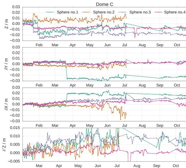
**Figure 5.** Evolution of the four reference spheres coordinates ( $x$ ,  $y$ ,  $z$ ) at Dome C.  $\delta$  and  $\delta'$  respectively refer to the changes with respect to the first scan (1 January 2015) and to a scan just after a period of settling (1 February 2015).
