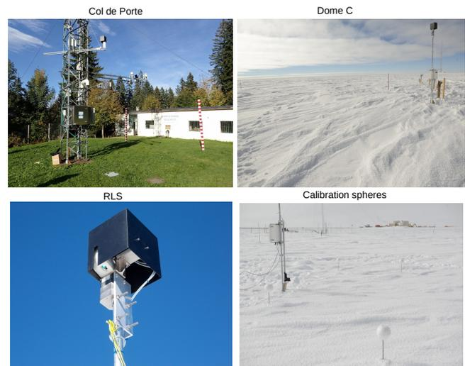
**Figure 2.** Pictures of RLS during the installation at Col de Porte (October 2014) and at Dome C (December 2014). Zoomed image of RLS (2-axis mount, laser meter and protection) and calibration spheres at Dome C.
