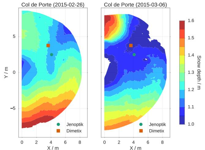
**Figure 8.** Two snow depth maps acquired at Col de Porte 26 February 2015 when the snow depth reaches its maximum and 6 March 2015 after a wind slab appeared in the northern corner ( $x = 0$ ;  $y = 6$  m). North is approximately in the  $y$ -axis direction. The square and round symbols represent the footprint of the SPICE sensors at the beginning of the season.
