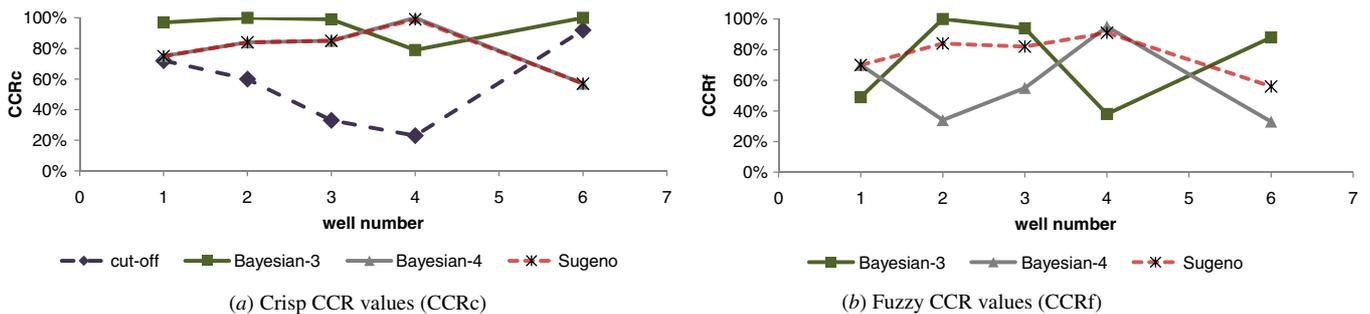
**Figure 7.** CCR of each methodology (conventional, Bayesian and fuzzy-based) in well no 1, 2, 3, 4 and 6. It was impossible to calculate the CCR in well no 5 due to lack of a valid well test. CCR values are calculated in two states: crisp and fuzzy.
