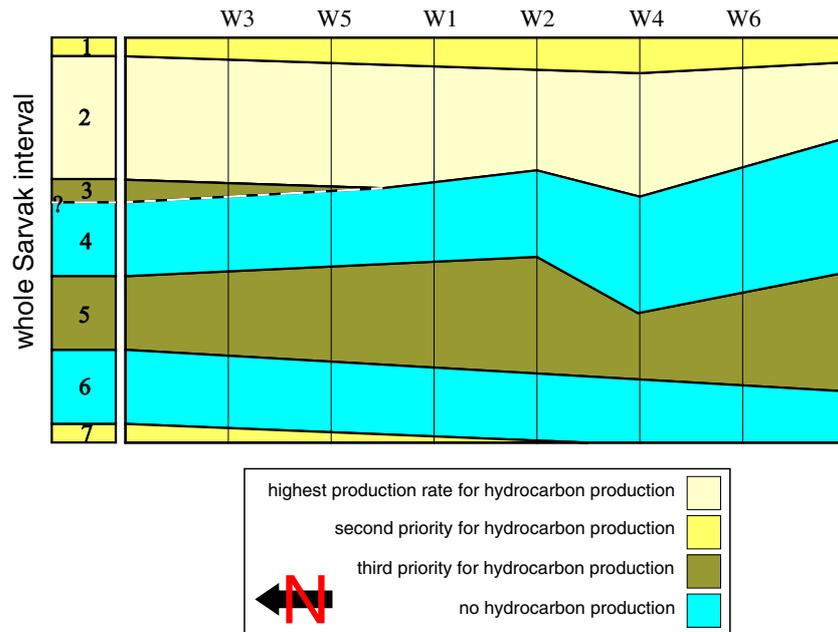
**Figure 8.** Final zoning for the productivity of Sarvak formation, resulted from integrating the outputs of different classification methods.
