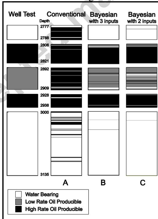
Figure 7: Results of three net pay determination procedures are compared with well test in training well. The track (A) is results of conventional cut-off-based method; track (B) shows results of Bayesian method with three input features (porosity, water saturation and shale content); and right track (C) reveals results of Bayesian method with two input features (porosity and water saturation).
