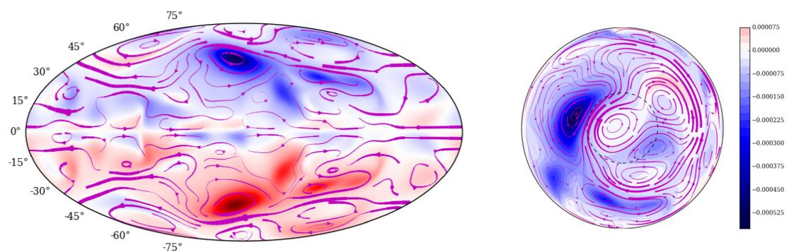
Figure 3: Growing radial magnetic field (colormap) and streamlines of the surface mean flow for  $Rm = 978$  and  $\Lambda = 0.9$ . **Left:** Aitoff projection at the core surface centered on the Pacific; **Right:** north-pole view projected onto the equatorial plane. The thickness of the streamlines is proportional to the velocity. The dashed circle marks the boundary of the Earth's inner-core.
