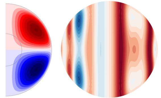
Figure 1: **Left:** the toroidal field  $\mathbf{B}_0$  that enters the magnetic pumping. **Right:** the flow distorted by the magnetic pumping (flow component perpendicular to the plane containing the axis).
