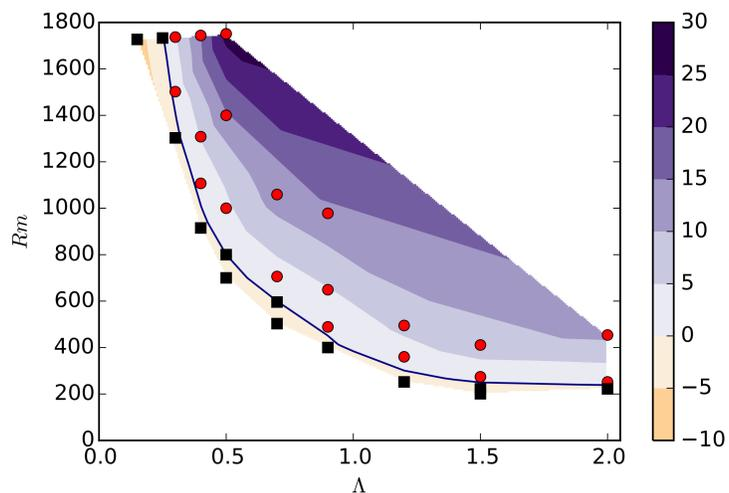
Figure 2: Growth rate (normalized by the magnetic diffusion time) as a function of the magnetic Reynolds number  $Rm$  and the Elsasser number  $\Lambda$  controlling the magnetic pumping. Black squares are failed dynamos (for which the magnetic field decays) while red circles are dynamos (exhibiting growing magnetic field).
