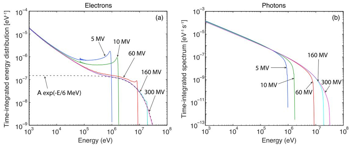
**Figure 3.** (a) Time-integrated electron energy distribution functions for each lightning leader potential drop magnitude used in the present study. (b) Corresponding bremsstrahlung photon spectra calculated using equation (2).
