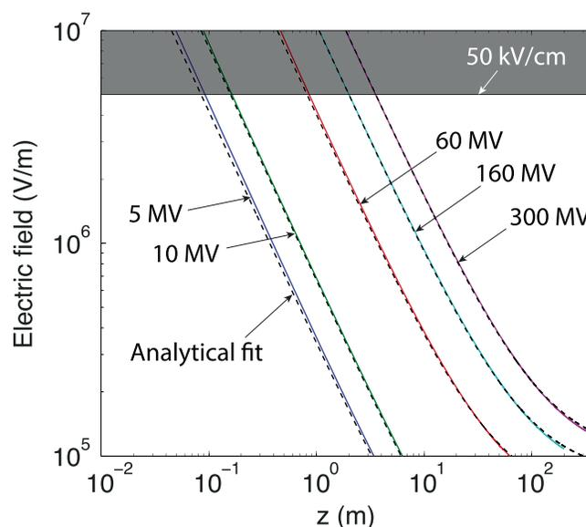
**Figure 1.** Electric field with respect to the distance from the leader tip calculated using the method of moments. The dashed lines represent analytical fits of the numerical solutions calculated using equation (1). Electric fields with amplitudes greater than 50 kV/cm are not considered in this study (grey area) as they could only be present on very short timescales. In the Monte Carlo simulations, electrons are injected at the location where the field is equal to 50 kV/cm.
