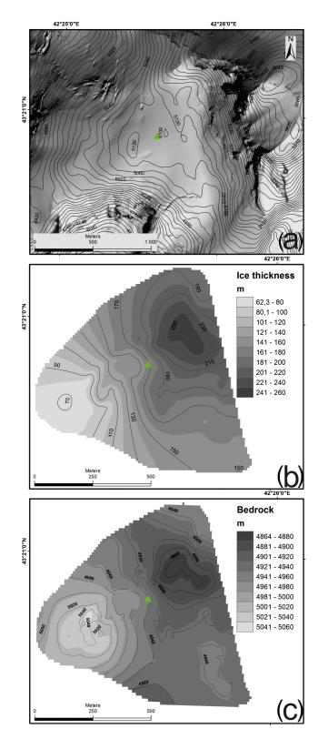
**Figure 4.** Glacier surface (**a**), ice thickness (**b**), and bedrock relief (**c**) on the western Elbrus plateau. The green triangle marks the position of the drilling site.
