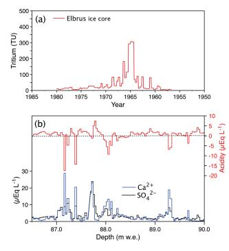
**Figure 10.** Absolute time horizons: (a) tritium measurements made on Elbrus ice-core samples (data were converted to 2009 with regard to the half-life time of tritium,  $T_{1/2} = 12.32$  year). The dates reported in the tritium curve are derived from the ammonium stratigraphy. (b) Calculated acidity (top; see Sect. 3.3.1), and calcium and sulfate (bottom) in ice layers located between 86.5 and 90 m w.e.
