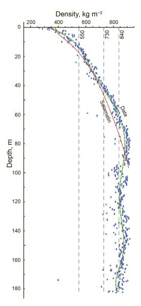
**Figure 5.** Measured (blue dots) and simulated (red line) ice-core density profile with critical densities shown as dashed lines (see Sect. 3.3.2). The green dashed line is a running mean for the measured density values.
