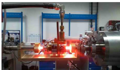
Fig. 1: the surfatron discharge in front of the VUV monochromator
