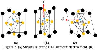
Figure 2. (a) Structure of the PZT without electric field. (b) Distortion of the structure with vertical applied field. (c) Distortion when othogonal field is applied.
