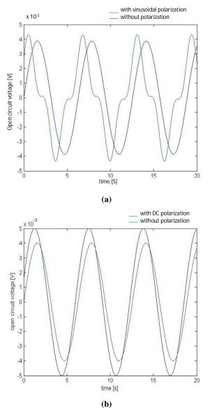
Figure 3. Open circuit voltage when a sinusoidal vertical acceleration, with a magnitude of 0,9 m/s<sup>-2</sup> and frequency of 50Hz, is applied to the cantilever
