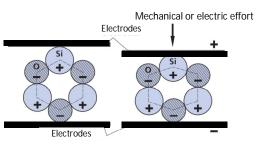
Figure 1. Cutting of an elementary cell of a quartz crystal under the effect of a mechanical or electric effort
