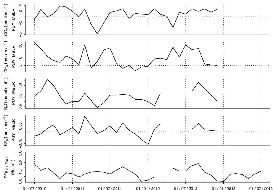
**Figure 7.** Differences between the monthly background at Puy de Dôme and the respective monthly MBLR (Dlugokencky et al., 2013a, b) at 45.5° N latitude for CO<sub>2</sub>, CH<sub>4</sub>, N<sub>2</sub>O and SF<sub>6</sub>. The last panel is the <sup>222</sup>Rn offset relative to marine air.
