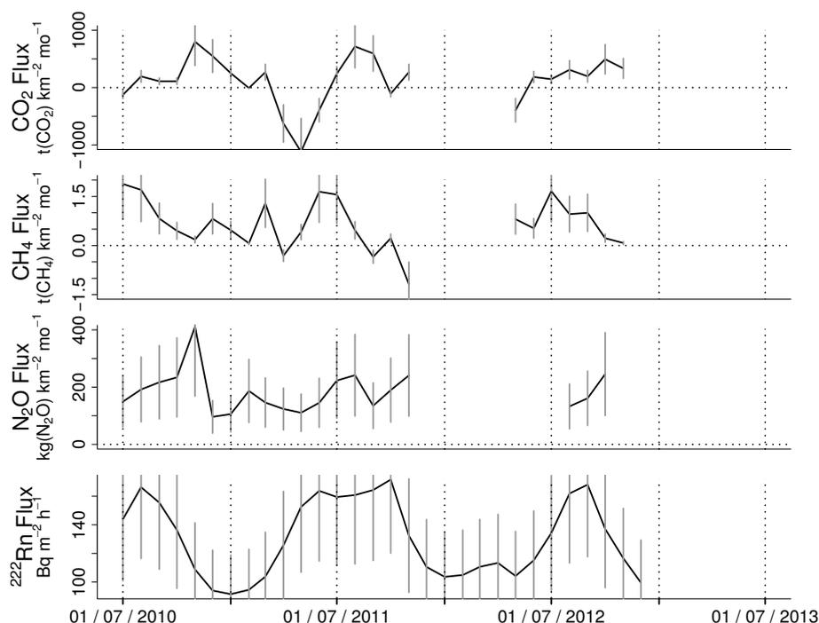
**Figure 8.** Monthly  $\text{CO}_2$ ,  $\text{CH}_4$  and  $\text{N}_2\text{O}$  fluxes at the Puy de Dôme station derived from the radon tracer method. The last panel presents the hourly  $^{222}\text{Rn}$  exhalation rate (U. Karstens and I. Levin, personal communication, 2014). The vertical grey lines are the respective flux uncertainties.
