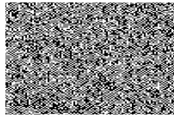
Figure 4 a). Start (1 Mc cycle), A: white, B: black, V: grey (A=B = 40%, V= 20%, \varepsilon_{AA}=\varepsilon_{AB}=\varepsilon_{AV} =0.6 ; \varepsilon_{BB}=\varepsilon_{BV} =0.4 )
