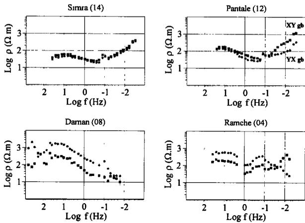
**Figure 3.** Components XY and YX of the decomposed MT transfer functions represented for four sites, Simra (14) and Pantale (12) in the south, Daman (08) in the Kathmandu valley and Ramche (04) in the north.
