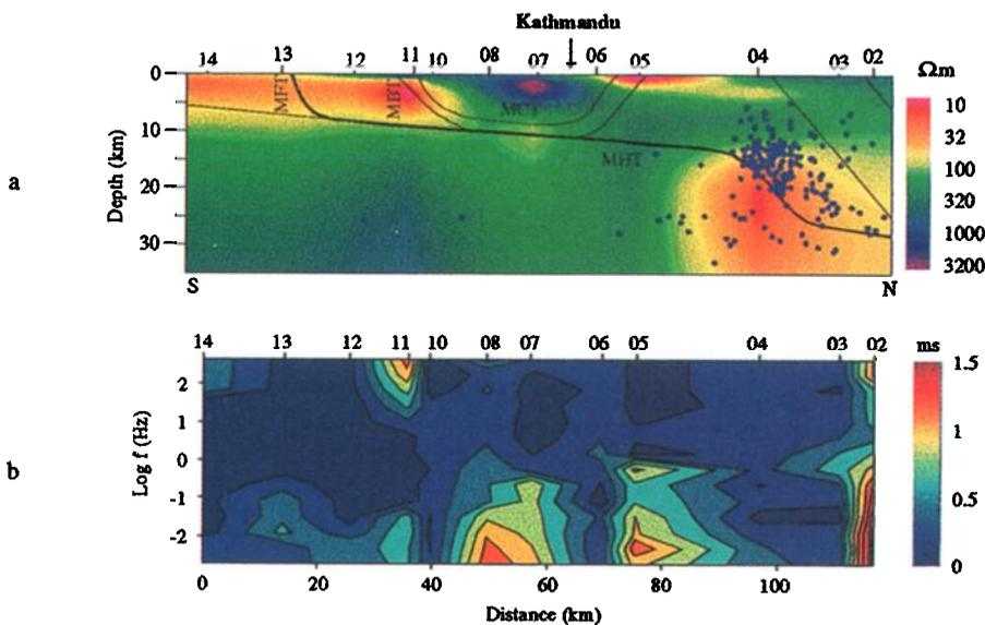
**Figure 4.** a) N20°E cross section of resistivity model derived from the 2-D inversion of MT data. Main Frontal Thrust (MFT), Main Boundary Thrust (MBT), Main Central Thrust (MCT) and Main Himalayan Thrust (MHT) are represented. Hypocenters within 30 km from the section recorded by the temporary seismic network (Figure 1) are shown in blue. b) Pseudosection illustrating the misfit between the model response and the observed data (see text). Site locations are plotted from south to north.
