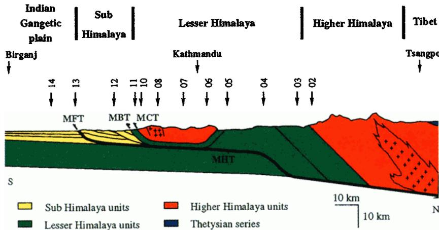
**Figure 2.** Geological section across the central Himalaya of Nepal (along the line through Birganj and Syabru-Bensi indicated in Figure 1) with MT site locations. Locations of major faults are shown. The thick line indicates the geometry of the main active fault (MHT) as inferred from structural geology and geomorphic evidence of uplift.
