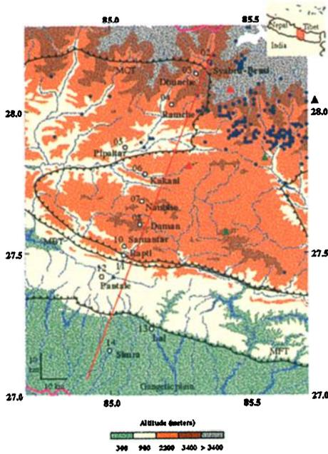
**Figure 1.** Topographic map of Central Nepal with locations of MT soundings (white dots) on (see insert for location in Nepal). The major faults, MFT (Main Frontal Thrust), MBT (Main Boundary Thrust) and MCT (Main Central Thrust) are also represented. The red line shows the location of section of Figure 2. Epicenters recorded from April to December 1995 by a network of temporary 3-cp stations (red triangles) and permanent 1-cp stations (green triangles) are indicated in blue.
