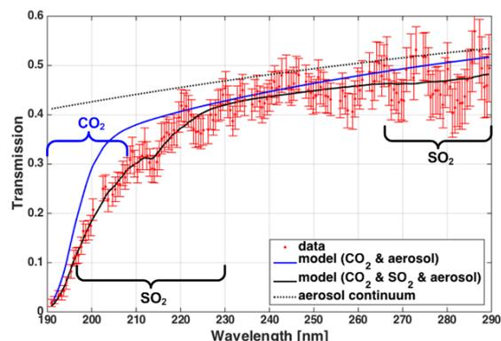
Fig. 1. An example of measured transmission spectrum (red dots with error bars) from a stellar occultation at altitude 90 km (orbit 1073, LT 2:00am, Lat 37.81°N). Molecular absorptions of CO<sub>2</sub> (in blue) and SO<sub>2</sub> (in black) are detected together with aerosol continuum (black dashed):  $N_{\text{CO}_2}=3 \cdot 10^{23} \text{ cm}^{-2}$ ;  $N_{\text{SO}_2}=8 \cdot 10^{16} \text{ cm}^{-2}$ .
