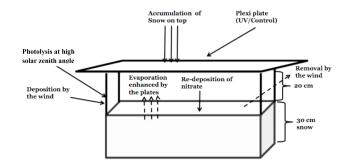
**Figure 9.** Schematic showing the possible external processes that could affect the surface layers of both the UV and control pits. These include evaporation, wind deposition and/or removal and photolysis at high solar zenith angle.
