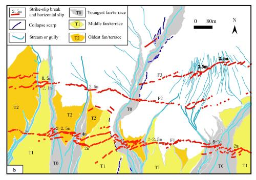
**Figure 15.** (a) Ikonos image created on 6 January 2003, around the site 93.365°E where *Lin et al.* [2002] gave a maximum coseismic horizontal displacement of 16.3 m. (b) Detailed strip map showing the surface rupture pattern of the Kunlunshan earthquake and coseismic horizontal displacements on different rupture strands. Blank areas are the pre-Quaternary of Kunlun Range.
