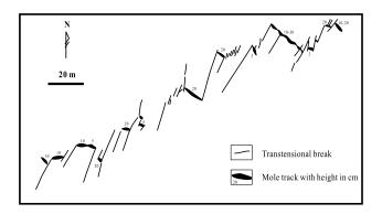
**Figure 3.** Measured terminal extensional structures for the 2001 Kunlunshan earthquake surface ruptures at the westernmost end of the western strike-slip section east of Kushuihuan Lake (35.959°N, 90.257°E).
