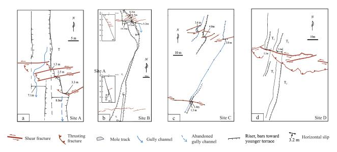
**Figure 13.** Measured topographic map showing surface rupture pattern and coseismic left-lateral and vertical displacements on the Yuxi Feng subsection (locations are marked in Figures 1b and 11). (a) Site A (35.767°N, 93.323°E). (b) Site B (35.767°N, 93.325°E). (c) Site C (35.762°N, 93.398°E). (d) Site D (35.814°N, 92.955°E).
