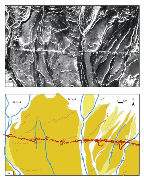
**Figure 16.** (a) Ikonos image created on 6 January 2003 that covers the area where *Lin et al.* [2002] gave a coseismic horizontal displacement of about 13.5 m. (b) Detailed strip map showing the surface rupture pattern of the Kunlunshan earthquake and coseismic horizontal displacements on different rupture strands. The legends are same as Figure 15.
