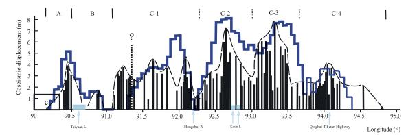
**Figure 14.** Distribution of the measured horizontal coseismic horizontal displacements along the strike of the surface rupture zone. Blue lines represent the coseismic horizontal displacements inferred from INSAR data [*Lasserre et al.*, 2005]. Other legends are the same as in Figure 1. Horizontal displacements are collected from *Xu et al.* [2002b], *Dang and Wang* [2002], *Chen et al.* [2003], and also measurements in the field.
