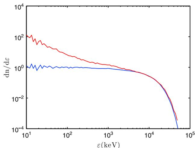
**Figure 10.** The energy distribution of RREAs simulated in an electric field of 400 kV/m. The red graph indicates the time-dependent simulation results, and the blue graph indicates the distance-dependent results.
