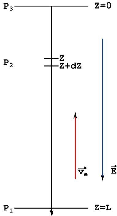
**Figure A1.** A schematic representation of a system where the electrons move with a velocity  $\vec{v}_e$  in an electric field  $\vec{E}$  and thus creating an avalanche in the region from  $Z = 0$  to  $Z = L$ . Three points of interest are also marked in the figure as points  $P_1$ ,  $P_2$ , and  $P_3$ .
