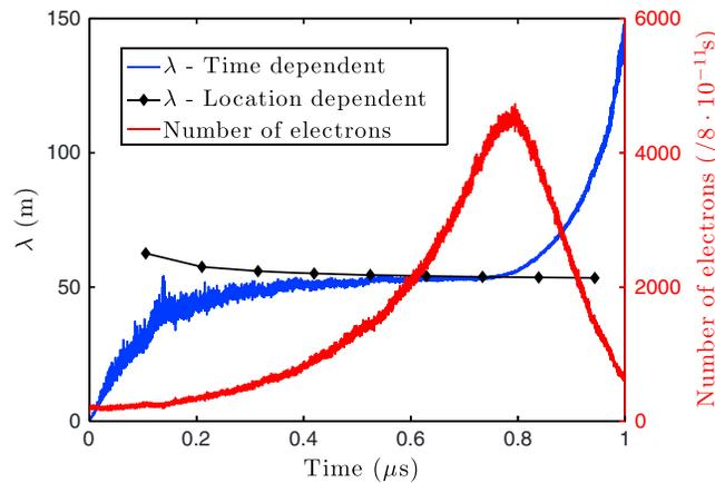
**Figure 2.** Electron multiplication with time (red line) and the corresponding avalanche lengths  $\lambda$  by time dependency (blue line) and location dependency (black line). The correlation between time and distance is given by the average speed of the developing avalanche of  $0.89c$  Coleman and Dwyer [2006]. This case was simulated using the LBE physics list.
