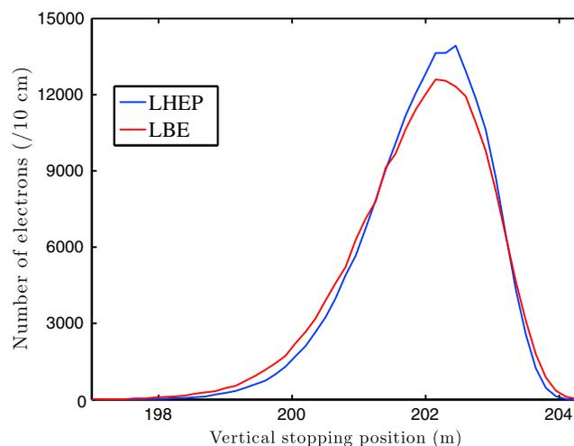
**Figure 9.** The stopping position of 50,000 electrons of 1 MeV per 10 cm without the influence of an electric field. The LBE results are indicated by the red color, and the LHEP results are indicated by the blue color. Note that the initial vertical position of the electrons is at 200 m.
