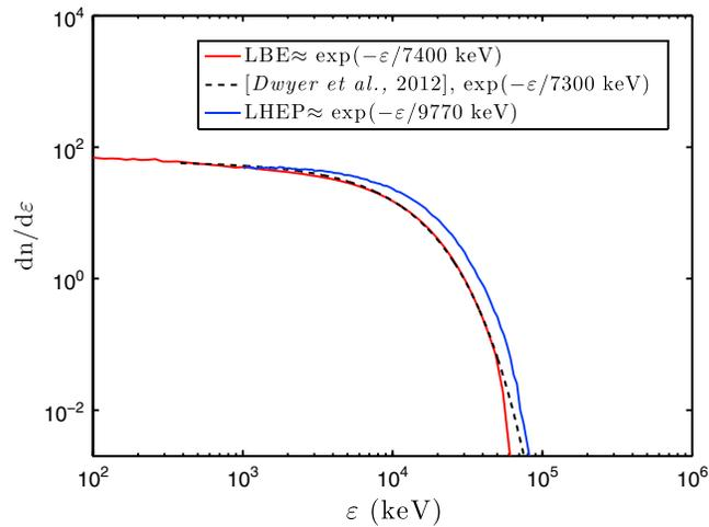
**Figure 4.** The electron energy distribution from simulations using the LBE physics list (red) and the LHEP physics list (blue). In addition, these results are compared to the exponential function  $\exp(-\epsilon/7300)$  found by Dwyer et al. [2012] (dashed black). Note that there is a deviation at very high energies where GEANT4 results do not follow an exponential cutoff.
