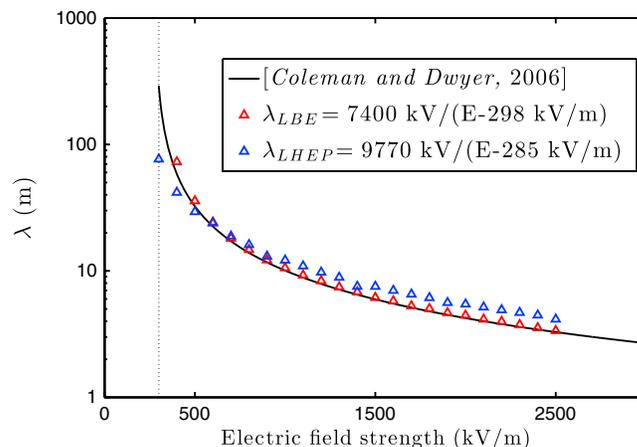
**Figure 3.** The avalanche length  $\lambda$  with respect to electric field strength. The LBE and LHEP results are marked as red and blue triangles, respectively. The continuous black line follows equation (6), which is the avalanche length determined by Coleman and Dwyer [2006]. In addition, the dotted black line marks the minimum electric field threshold  $E_{\text{th}} = 284 \text{ kV/m}$ .
