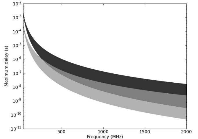
**Fig. 6.** These curves show the upper limits on the size of delays from second-order ISM effects extrapolated up to higher frequencies. The dark grey area is for PSR B0809+74, which had the largest RMS residuals in our timing fits; the light grey area is for PSR B1919+21, which had the smallest RMS residuals. They are scaled with  $\nu^{-3}$  and  $\nu^{-4}$  which are the lower and upper bounds for scaling of the second-order ISM effects.
