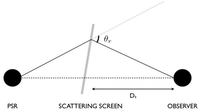
**Fig. 8.** A gradient in the electron density perpendicular to the line-of-sight causes rays to be bent. The size of the angle which the rays are bent through depends on the frequency of the radiation. Low frequencies (dark line) are bent through a larger angle and so must travel along a longer path to reach the observer, delaying them with respect to higher frequencies (dashed line).
