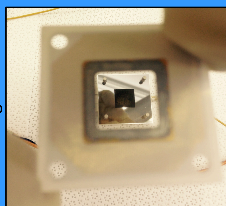
Fig. 2 15 mm 2 CNT chip in the lens of the G1 grid grounded at +OV.
