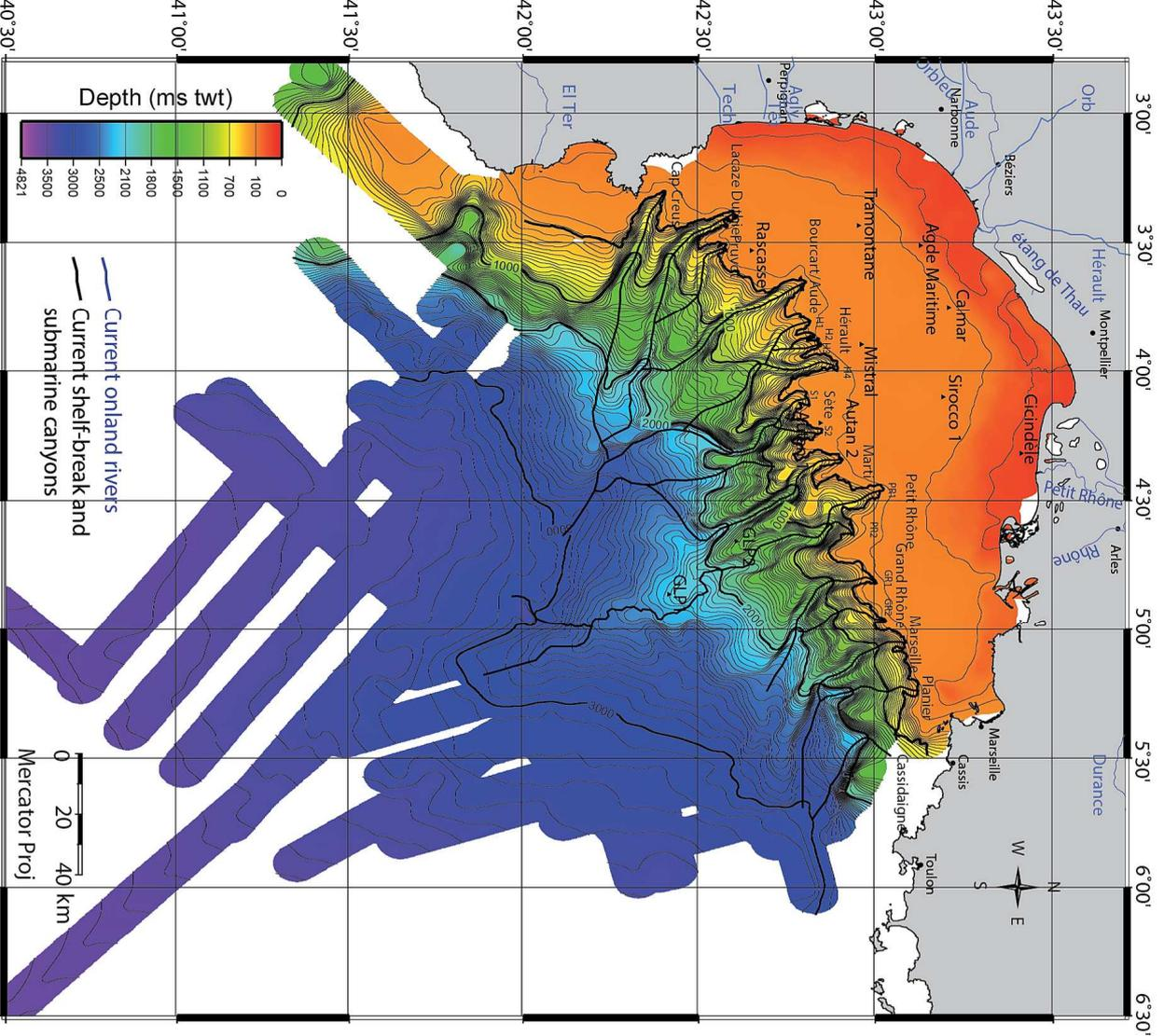
Isobaths (ms twt) of the seafloor from our seismic data
