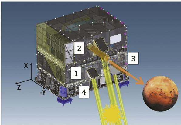
**Fig. 1.** The NOMAD instrument, with the SO (1), LNO (2) and UVIS (3) channels, and the electronics (4). Lines of sight towards the Sun (yellow cylinders) and the nadir direction (orange cylinders) are also indicated. (For interpretation of the references to color in this figure legend, the reader is referred to the web version of this article.)
