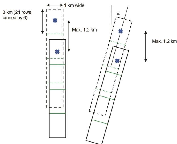
**Fig. 9.** Representation of a perpendicular and off-perpendicular slit of the SO channel (not to scale): in dashed line at time  $t_0$  and in plain at time  $t_0 + 1$  s, considering a 1 s cycle and a maximum downward velocity of 1.2 km.
