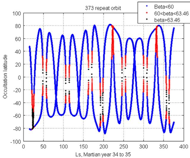
**Fig. 7.** Latitude of occultations over 1 Martian year for various beta angles. It is clear that being able to observe the red marked occultations between beta angles 60 and 63.46 would greatly increase the NOMAD coverage.
