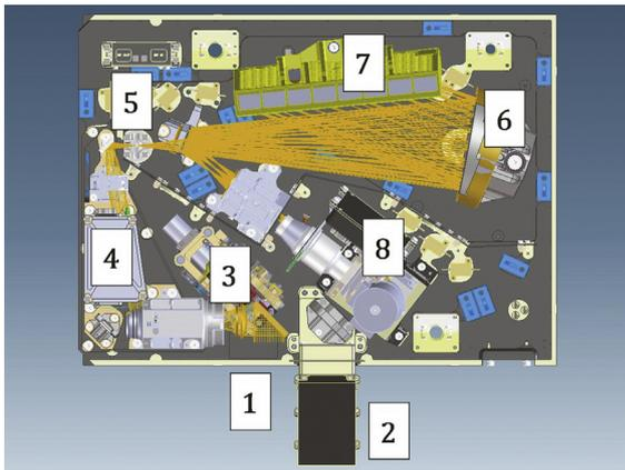
**Fig. 3.** View of the LNO channel and its components: (1) the entrance optics, (2) the solar occultation periscope, (3) the flip-mirror mechanism, (4) the AOTF filter, (5) the spectrometer entrance slit, (6) the folding mirror, (7) the echelle grating, (8) the detector.
