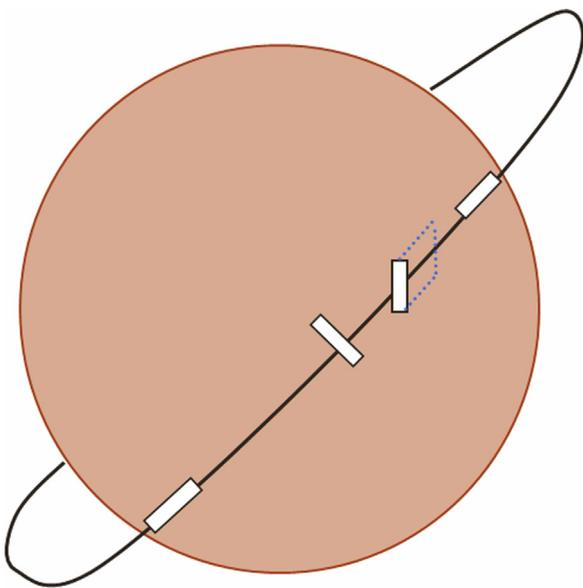
**Fig. 11.** A representation of the evolution of the slit angle w.r.t the ground track for beta angle  $=0^\circ$ . The blue dashed parallelogram shows the area swept out during an integration time. This image is not to scale. The view is from the Sun, the disk is then the day side of the planet, and the circle circumference is the terminator.
