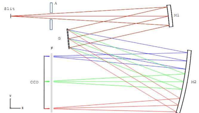
**Fig. 4.** Schematics of the UVIS instrument: the entrance slit (Slit), the aperture (A), the collimating mirror (M1), the diffraction grating (G), the focusing mirror (M2), the 2nd order filter (F) and the detector (CCD).
