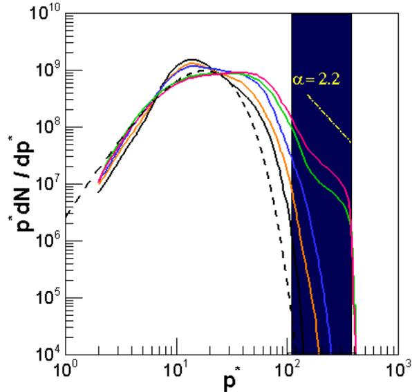
Fig. 4.— The electron spectrum taken at  $200\lambda_{ce}$  within the RS transition region from  $t^* = 420$  (leftmost solid black line) up to 500 (rightmost solid red line) with an interval of  $\Delta t^* = 20$  ( $200\lambda_{ce}$  is calculated relative to the RS position at each time). The dashed line shows a 3D Maxwell-Jüttner distribution. Dashed-dotted line shows a power-law fit to the non-thermal component in the electron energy spectrum at the latest time.
