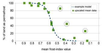
**Figure 10.** Frost-index-predicted permafrost fraction of land from Fig. 8 upscaled to the CLIMBER-2 grid and plotted against mean frost index for the same CLIMBER-2 grid cell. Circled points are where the total fraction of land vs. ocean in the grid cell is small (land is less than 25% of the grid cell) and ocean temperatures pull frost index lower (warmer). The dashed line is a representative relationship between frost index and permafrost land fraction.
