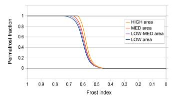
**Figure 11.** CLIMBER-2P model for permafrost fraction of the land in a grid cell from frost index (snow corrected). Range of areas is within the range of estimates for present-day land area underlain by permafrost by Zhang et al. (2000). Permafrost fraction is limited between 0 and 1. Zhang estimate for total permafrost area is 12.21 to  $16.98 \times 10^6$  km<sup>2</sup>. Listed from HIGH to LOW, model output is 16.35, 14.87, 14.00 and  $13.21 \times 10^6$  km<sup>2</sup>.
