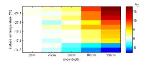
**Figure B2.** Model error when the linear snow correction model is used to predict temperatures at snow-depth or snow–ground interface for data from Morse and Burn (2010) (measurement data are down snow column temperatures). Positive numbers indicate that the linear model output is too warm compared to data.
