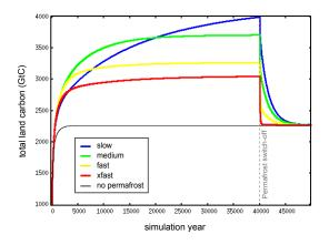
**Figure 13.** Total land carbon (GtC) for the PI(eq) simulation followed by a permafrost switch-off at 40 k simulation years representing a complete and immediate permafrost thaw, demonstrating the different dynamic behaviour of each dynamic setting.
