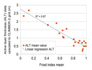
**Figure 7.** Measurement data for active layer thickness (CALM network, Brown et al., 2003) and frost index (Zhang, 1998) upscaled to the CLIMBER-2 grid scale, showing the distinct relationship of reducing active layer with increasing frost index at this scale. Note that permafrost fraction is calculated from frost index in our model (see Sect. 3.2).
