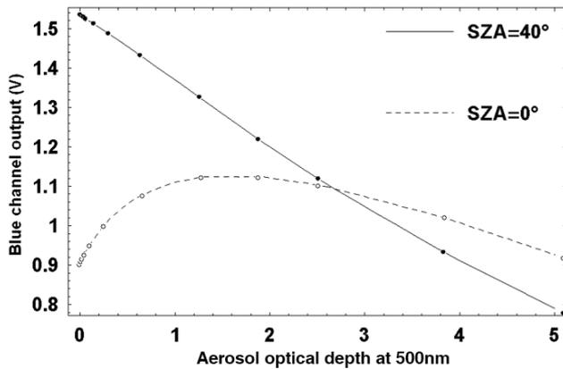
**Figure 1.** Solar flux received by ODS in the blue wavelength range as a function of the aerosol optical depth (AOD), at  $40^\circ$  SZA (solid line with black circles) for total direct and scattered sunlight and at  $0^\circ$  SZA (dashed line with white circles) for scattered sunlight only. The ratio between the two fluxes varies monotonously, with AOD providing a direct AOD measurement independent of sensor calibration.
