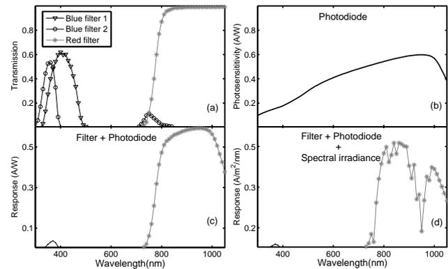
**Figure 3.** (a) Blue- and red-filter transmission. (b) Photodiode spectral response. (c) Response of filters–photodiodes combination. (d) Final blue-channel response ( $370 \mu\text{m} \pm 20 \mu\text{m}$ ) on the left and red-channel response ( $902 \mu\text{m} \pm 169 \mu\text{m}$ ) on the right.
