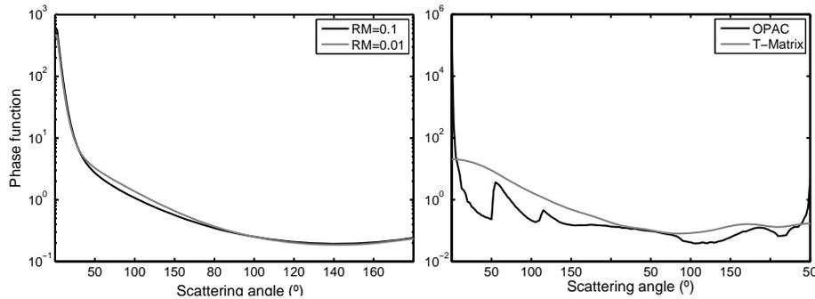
**Figure 9.** (a) Phase functions at 370 nm calculated by the empirical formulation proposed by Pollack and Cuzzi assuming a bimodal size distribution. The phase functions are calculated for two different ratios between modes. (b) Phase functions at 902 nm derived from the OPAC software and T-matrix method for cloud particles.
