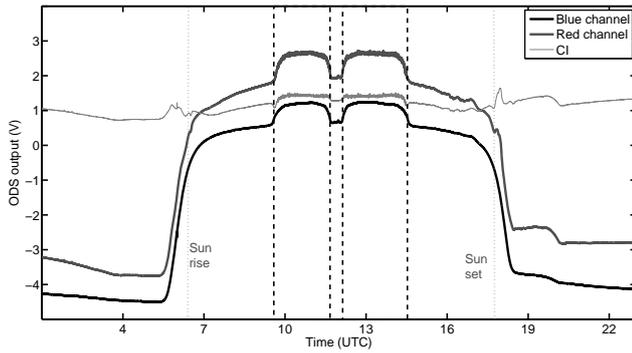
**Figure 4.** ODS measurement in Ouagadougou on 23 December 2004 in cloud-free conditions. The bands delimited by the black dashed lines represent the time intervals for which the sun is within the FOV of ODS.
