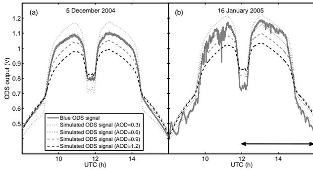
**Figure 8.** Comparison between ODS blue channel observed output voltage and simulated blue ODS signal for AOD values of 0.1, 0.6 and 1 (a) in cloud-free conditions on 5 December 2004 and (b) on 16 January 2005 in cloudy conditions.
