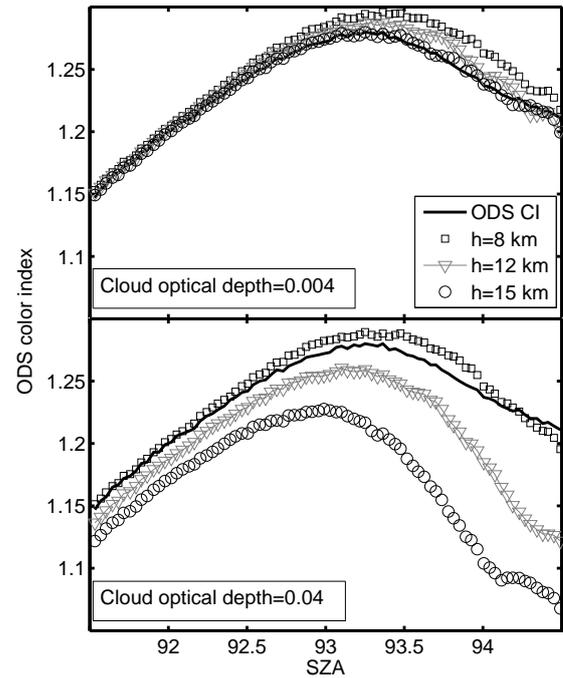
**Figure 10.** (a) ODS color index (black solid line) during sunset for one day of the campaign and simulated color index for COD = 0.004 and cloud altitude  $h = 8, 12$  and  $15$  km. (b) Same as (a) but for COD = 0.04. The simulated CI for COD = 0.004 and  $h = 15$  km fits better with the ODS-measured CI.
