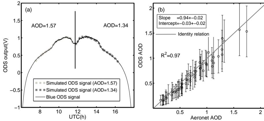
**Figure 15.** (a) Evolution of ODS signal measured on 5 January 2005 and those simulated for the AOD values obtained by the retrieval procedure of dust opacity using only half of the day. (b) Correlation between ODS blue channel and AERONET AOD at 370 nm for cloud-free days, and where two values of AOD per day have been estimated for days with a daily average AOD above 0.8.
