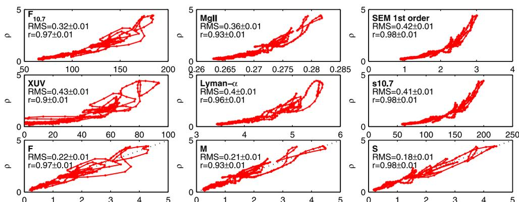
**Figure 2.** Scatter plot of the DC component of the thermospheric density versus the DC component of various solar inputs. The RMS and Spearman's correlation coefficient  $r$ , together with their standard deviation, are indicated for each proxy. The standard deviation has been obtained by bootstrapping. In all plots, a linear model  $\hat{\rho}_{DC} = \alpha + \beta x_{DC}$  is used for computing the RMS. Densities are in units of  $[10^{-14} \text{ kg m}^{-3}]$ .
