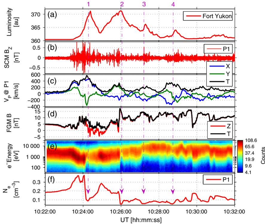
**Figure 1.** THEMIS data on 17 March 2008 between 10:22:00 and 10:32:00 UT: (a) total luminosity observed by the all-sky imager at Fort Yukon, (b) Z-component of the magnetic field oscillations from SCM, (c) X-, Y-, and total component of the ion velocity from ESA, (d) Z-, and total component of the magnetic field from FGM, (e) electron energy spectrogram, and (f) electron density from ESA at P1.
