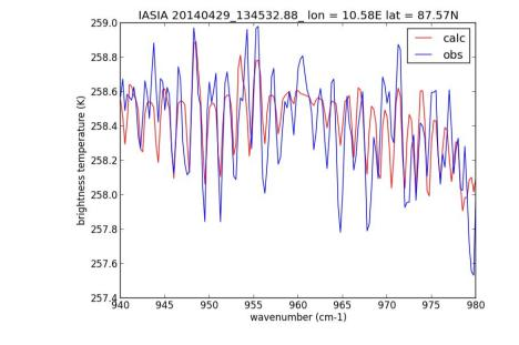
Figure 11 : Comparison between measured (blueline) and calculated (in red) Brightness Temperature at the Top-of-theatmosphere
