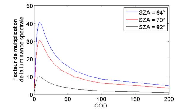
Fig. 7 Modelled Amplification Factor (MAF) of spectral luminance at the bottom of the atmosphere computed with MOMO against cloud optical depth (COD) for several solar zenith angles.
