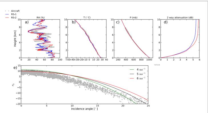
Two radiosondes were available before and after the 1:30 hour flight, Figures a, b, c represent the relative humidity, temperature and pressure profiles respectively. These profiles are used to calculate the two way attenuation at 94 GHz presented in panel d. Note that HYMEX and MT-Maldives system configurations were similar and therefore we use the same calibration constants.
