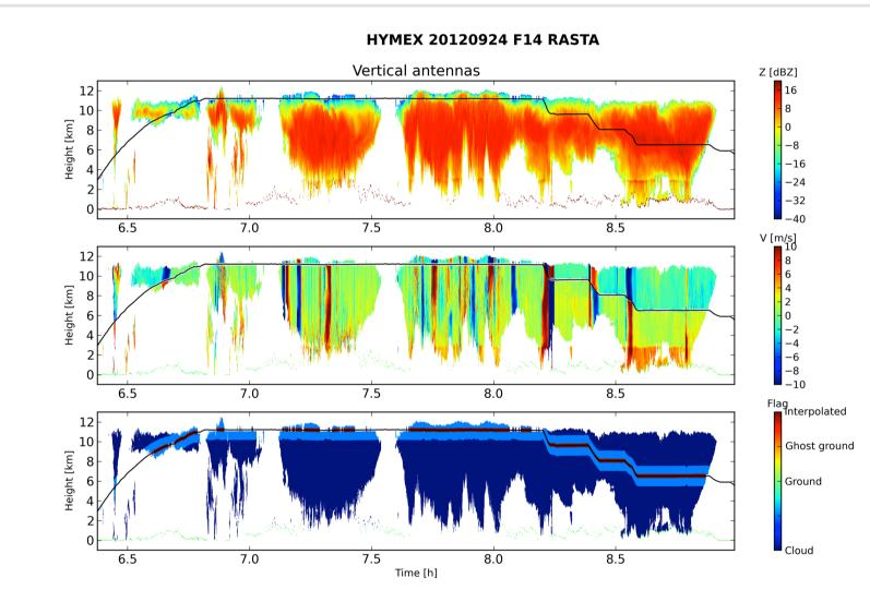
• Bottom panel shows the classification of the data (cloud, ground, interpolated reflectivity at aircraft altitude...)
