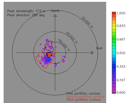
Figure 2: Directional sea wave slope spectrum obtained from a 30 s sample of KuROS observations. The ambiguity in the propagation direction has been removed using method 1. Energy density is in colour code, North-south and East-West wave number components are vertical and horizontal axis, in the meteo-oceanic convention.
