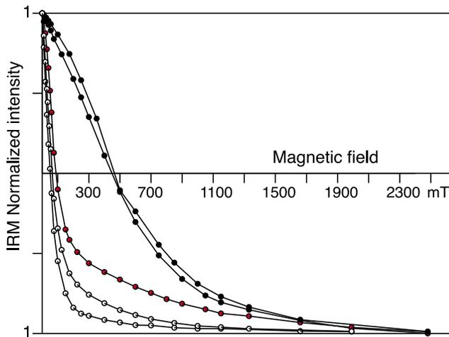
**Figure 3.** Backfield Isothermal Remanent Magnetization (IRM) acquisition after saturation with a field of 2500 mT. Black circles correspond to two samples from the Lower Kayra formation showing hematite as the main magnetic carrier. White circles correspond to two samples in the Soncco formation with magnetite and hematite as the magnetic carriers. Red circles correspond to a sample of the Kayra formation after heating in air in the laboratory up to 680°C with formation of magnetite.
