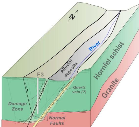
Fig. 1: Block diagram showing the aquifer situation.
