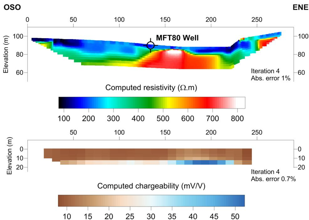
Fig. 2: Saint-Brice. a) Computed resistivity (Wenner-Schlumberger array, inter-electrode spacing = 3m).
