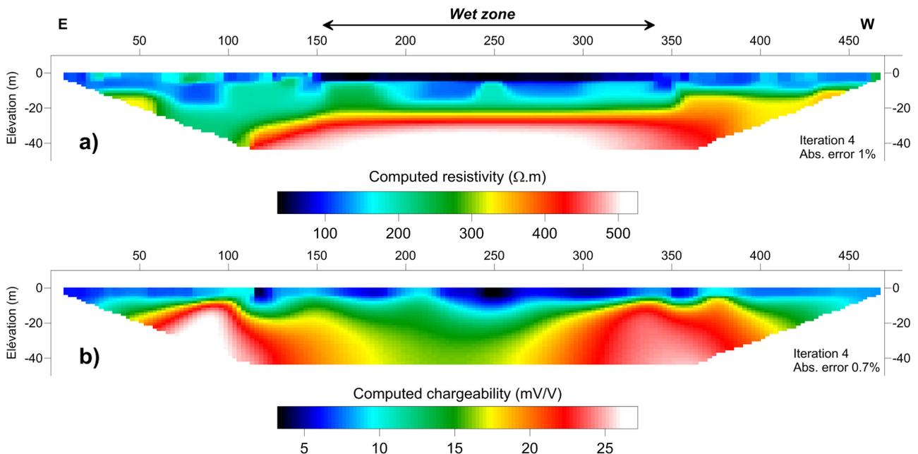
Fig. 4: Guidel (Wenner-Schlumberger array, inter-electrode spacing = 5m).
