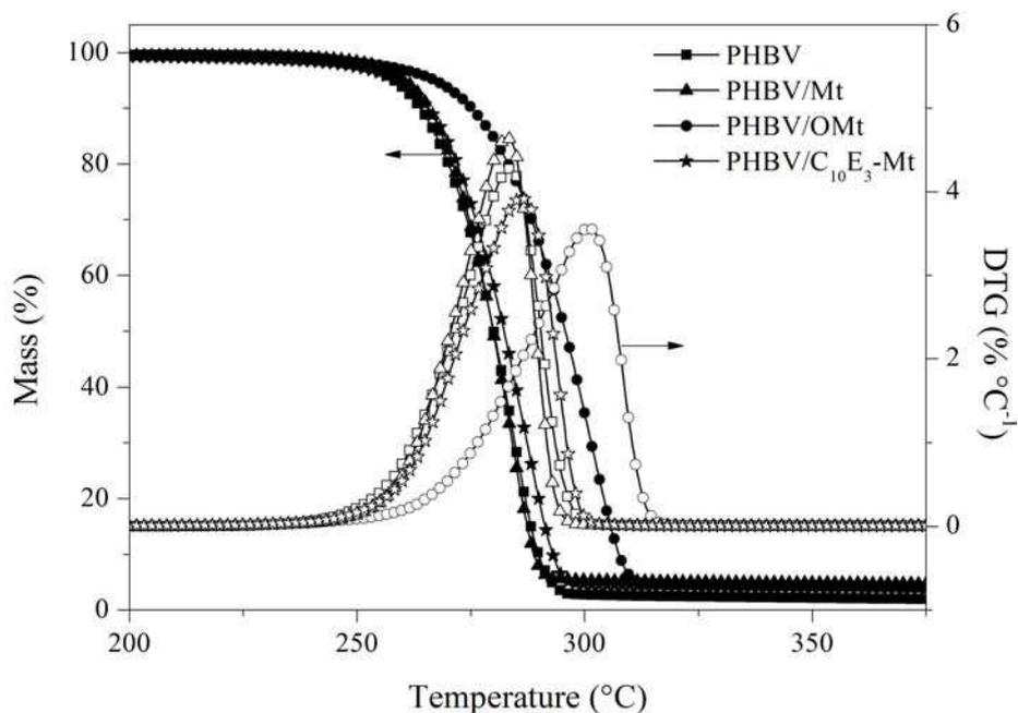
**Figure 5.** TGA and DTG curves of PHBV and PHBV nanocomposites (temperature error:  $\pm 0.5$  °C; mass error: 0.6%).
