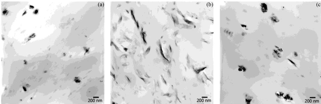
**Figure 2.** TEM micrographs of (a) PHBV/Mt, (b) PHBV/OMt, and (c) PHBV/C<sub>10</sub>E<sub>3</sub>-Mt nanocomposites.
