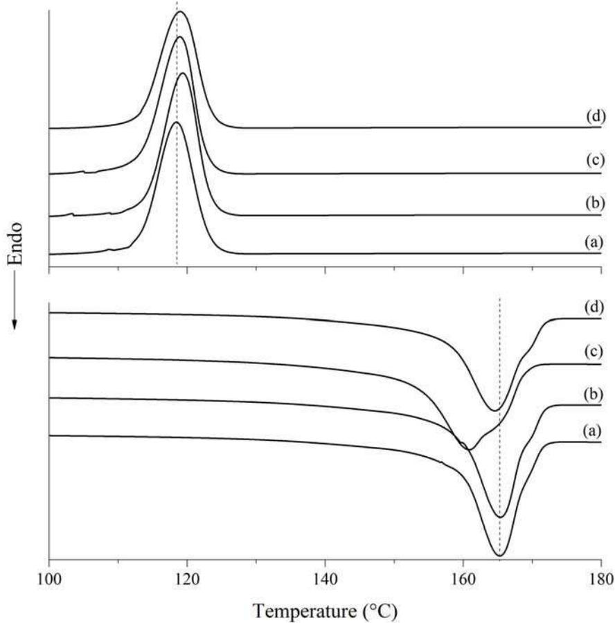
**Figure 4.** DSC curves of (a) PHBV and (b) PHBV/Mt, (c) PHBV/OMt, and (d) PHBV/C<sub>10</sub>E<sub>3</sub>-Mt nanocomposites (temperature error:  $\pm 1.0$  °C).
