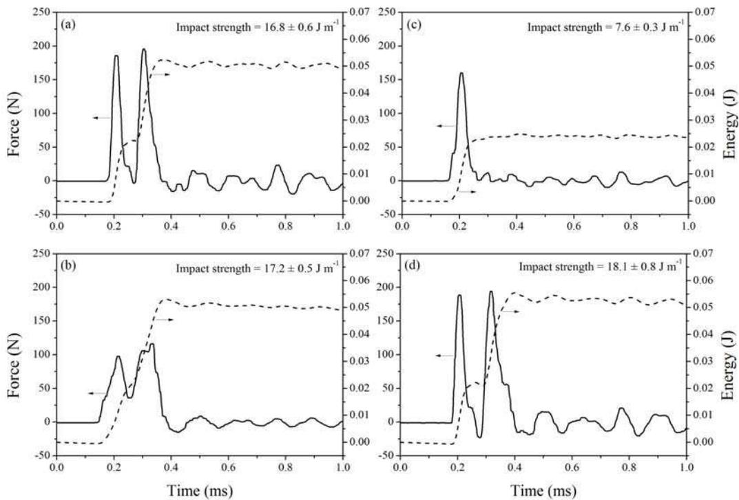
**Figure 7.** Force and absorbed energy vs. time curves of (a) PHBV, (b) PHBV/Mt, (c) PHBV/OMt, and (d) PHBV/C<sub>10</sub>E<sub>3</sub>-Mt nanocomposites from the instrumented impact tests.
