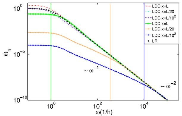
**Figure 3.** Head FTF  $\Theta_h(\omega)$  at different observation points for the LR, LDD, and LDC models. The vertical lines indicate the characteristic frequencies  $\omega_x=T/(x^2S)$  for the observation points (from left to right)  $x=L$ ,  $x=L/20$ , and  $x=L/10^2$ . We used:  $S=10^{-4}$ ,  $T=10^2$  m<sup>2</sup>h<sup>-1</sup>,  $\alpha_c=10^{-4}$  h<sup>-1</sup>, and  $L=10^3$  m. The aquifer response rate is  $\omega_L=1$  h.
