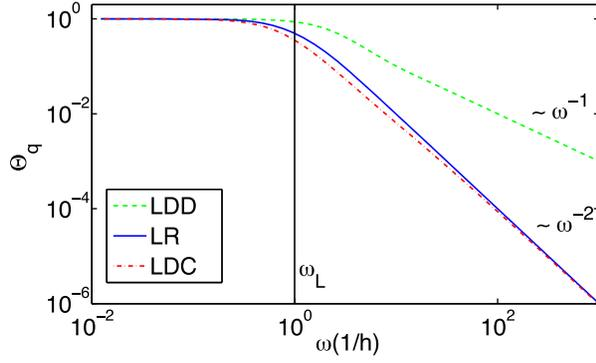
**Figure 2.** Discharge FTF  $\Theta_q(\omega)$  for the (dashed) LDD, (dash-dotted) LDC, and (solid) LR models. The vertical line indicates the aquifer response rate  $\omega_L=1$  h which is given by  $\omega_L=T/(L^2S)$  for the LDD and LDC models, and by  $\omega_L=\alpha/S$  for the LR model. We used  $S=10^{-4}$ ,  $T=10^2$  m<sup>2</sup>h<sup>-1</sup>,  $L=10^3$  m, and  $\alpha=\alpha_c=10^{-4}$  h<sup>-1</sup>.
