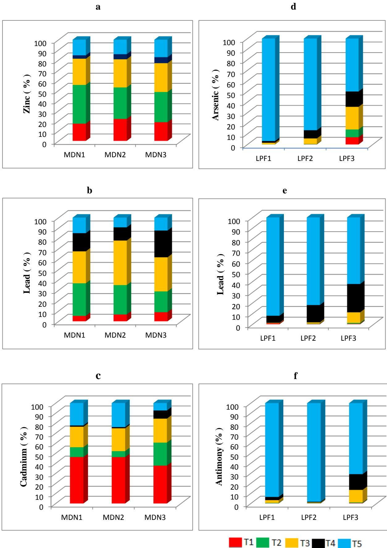
**Fig.1:** Chemical distribution of Zn (a), Pb (b and e), Cd (c), As (d), Sb (f) in the different soil fractions in MDN and LPF (Tessier's scheme): T1 (exchangeable), T2 (carbonates), T3 (reducible), T4 (oxidizable), T5 (residual).
