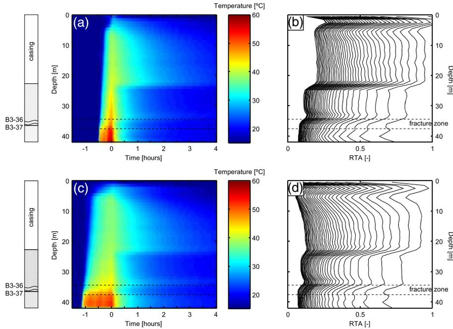
**Figure 2.** Temperature in B3 during the thermal dilution test under (a) ambient conditions and (c) while pumping B2, and (b) corresponding Relative Temperature Anomaly and (d) at normalized times of 0.2 to 8 [-] (right to left). The time was normalized to account for the different injection durations, with 1 h taken as the standard injection length.
