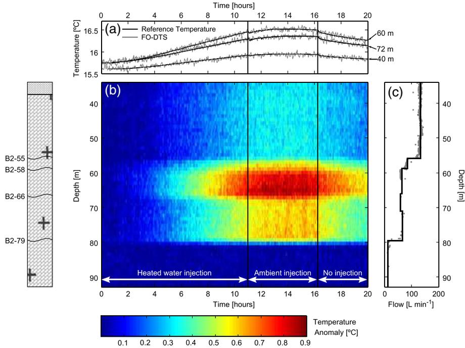
**Figure 3.** (a) Temperature logger and DTS measured temperature at the corresponding depths during the thermal tracer test from B1 to B2, (b) DTS measured temperature anomaly for all depths, and (c) measured flow in B2 for a pumping rate of  $140 \text{ L min}^{-1}$  with solid line to indicate the flow profile assumed for the application of equation (3).
